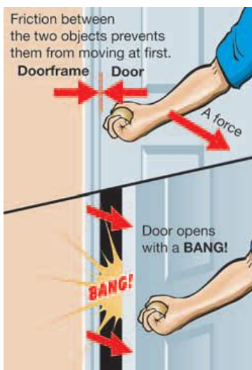
Figure 12.3: A stuck door is an example of stick-slip motion.
